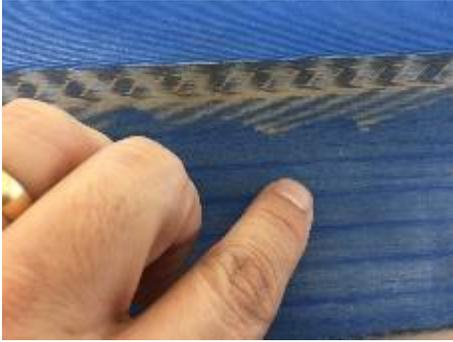
*The FFF 3D-printed PLA piece has an acceptable surface finish with only minimal filling and sanding required.*
