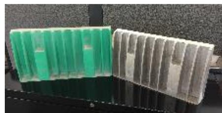
*3D printed PLA piece at left, aluminum casting at right.*
