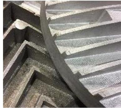
*On the right is the 3D-printed PLA piece, with the first run aluminum casting on the left.*
