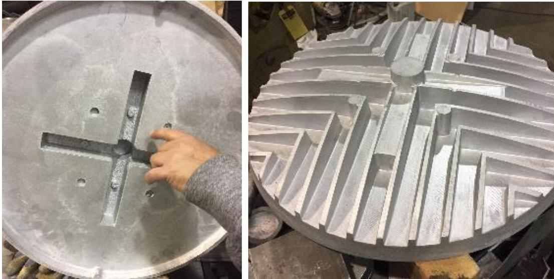
*The large format of the 3D Platform printer allows for the creation of parts that could not be printed using previous methods. This 0.53m (21") diameter printed master easily fit on the 1m x 1m (39" x 39") print bed. [All Image Source: U.S. Architectural Lighting]*
